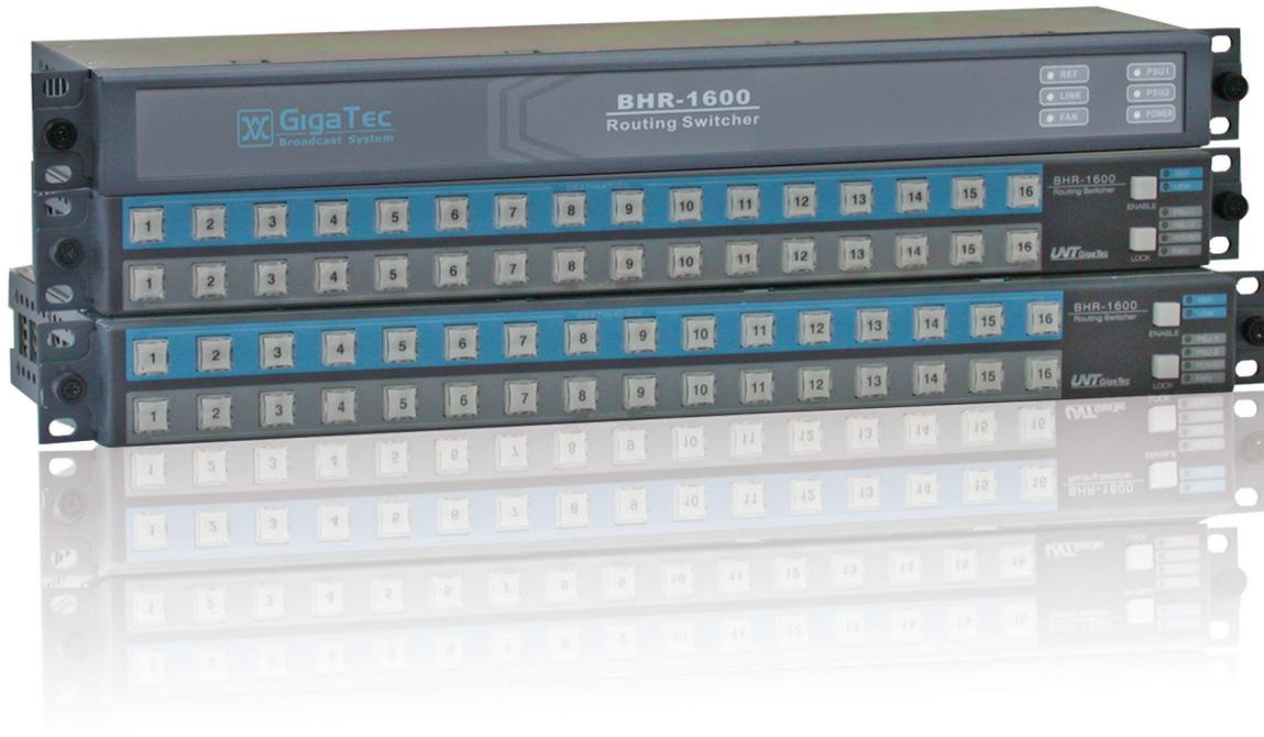
The BHR-1600 is a compact and cost-efficient routing switcher for 3G/HD/SD-SDI signals. Switching size is up to 16x16. Auto reclocking for signals at 270 Mbps, 1.483/1.485 Gbps or 2.976/2.970 Gbps is supported. Switching takes place at the vertical blanking interval for quality video and audio switch.
